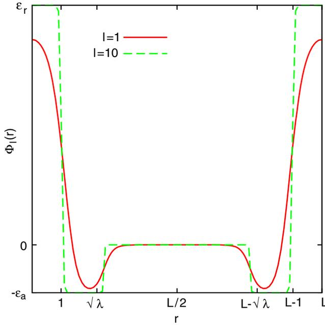
**Figure 1.** The potential  $\Phi_l(|x|)$  for  $L \gg 1$ . In the plot we used  $\epsilon_r = 5, \epsilon_a = 1, \Delta = 4$ , and  $L = 10$ , at two values of the smoothing parameter  $l$ .
