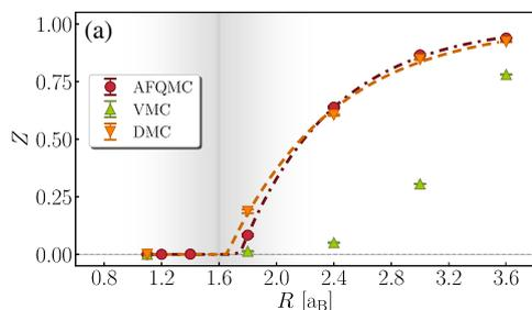
Figure 7.6: Metal-insulator transition in H-chains:  $|\mathfrak{z}_N|$  as a function of the interatomic distance  $R$  for different correlated wavefunctions at  $N = 40$ . The plot indicates a transition  $R$  value of 1.70 bohr. After Ref. [188].
