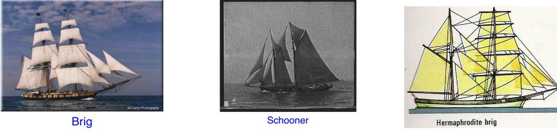
Figure 8.4: Two-masted vessels. Brig: both masts are square rigged. Schooner: both masts are fore-and-aft rigged (gaff sails and topsails here). Hermaphrodite brig: the foremast is square rigged, the mainmast is fore-and-aft rigged.
