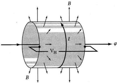
Figure 2.10: Geometry for Laughlin's Gedankenexperiment. A 2d channel is bent into a loop of circumference  $L$ , and a magnetic  $\mathbf{B}$  field of constant magnitude pierces the cylinder normal to the surface. A current  $I \equiv I_x$  circles the loop;  $V_H \equiv V_y$  is the Hall voltage. The loop may be threaded by the inaccessible flux  $\varphi$ .
