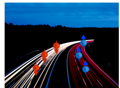
Fig. 2: The topological quantum “information highway”, representing the 1D dissipation-less transport at the edge of a 2D topological insulator, where electrons with opposite spins travel in opposite directions without scattering.
